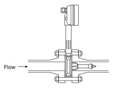
Fig. 8 Horizontal flow limited to 7 bar g
