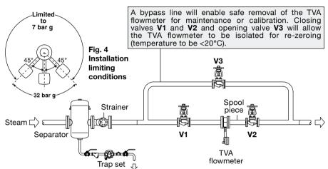
Fig. 5 Typical installation
