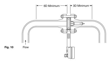
If any of the following configurations are present upstream of the TVA flowmeter:
