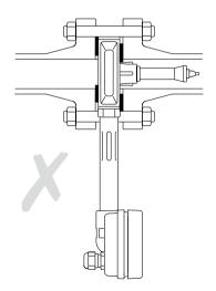
Fig. 16 Gaskets fitted incorrectly
