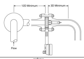
Avoid installing the TVA flowmeter downstream of an actuated valve as rapid cycling of the valve could give rise to inaccurate results or damage the flowmeter. See Figure 12. In configurations where there is more than one rapid acting pressure reducing valve close coupled, the TVA flowmeter should be installed with a minimum of 25 upstream and 3 downstream pipe diameters away from the valves.
