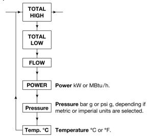
The following chart indicates the run mode data display sequence. Depending on the configuration, the flow units will be:
