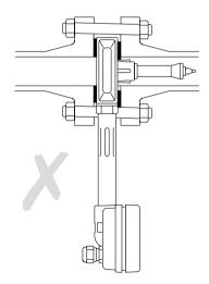
Fig. 17 Gaskets and pipe offline, fitting incorrectly
