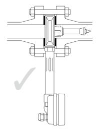
Fig. 15 Gaskets fitted correctly
