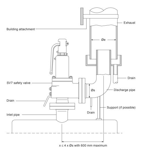
Fig. 5 Typical installation
