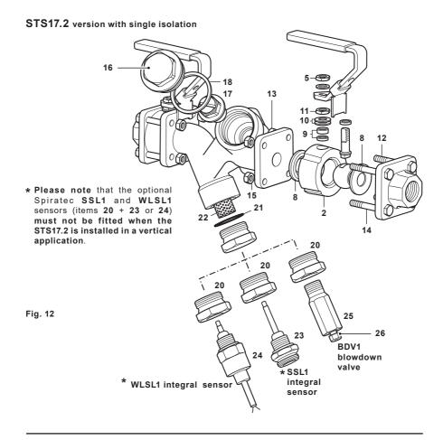
STS17.2 Stainless Steel Compact Pipeline Connector Steam Trapping Station
