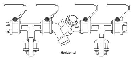
Fig. 4 Double Block and Bleed Upstream Horizontal Downstream Horizontal (DBB USH DSH)
