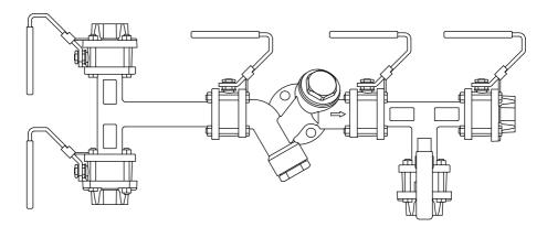
Fig. 6 Double Block and Bleed Upstream Vertical Downstream Horizontal (DBB USV DSH)
