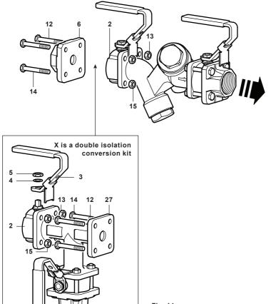
Fig. 14 How to fit a Double Block and Bleed conversion kit to a single isolation STS17.2
