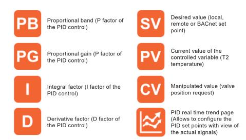
The following screen is accessible from above PID Loop Set Points page (available only for engineers). We are able to switch between proportional band and proportional gain. Trend shows us PID loop real time responses. The SV, PV and CV values at PID Real Time Trend are scaled to percent.
