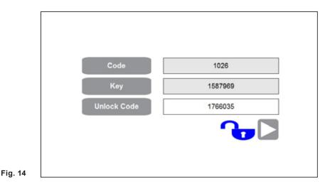
To be able to move to next page the unlock code is essential, which can be found on the authentification certificate supplied with the panel. After entering the proper code, the lock and the continue button will appear when pressed and transfer you to the time/date setting page.
