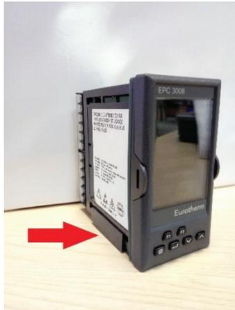
Fig. 10 Plastic holder to be removed
