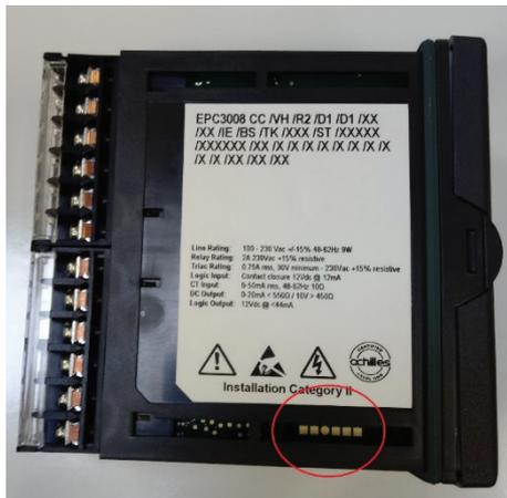
Fig. 11 Connection point of the CPI Clip-on connector
