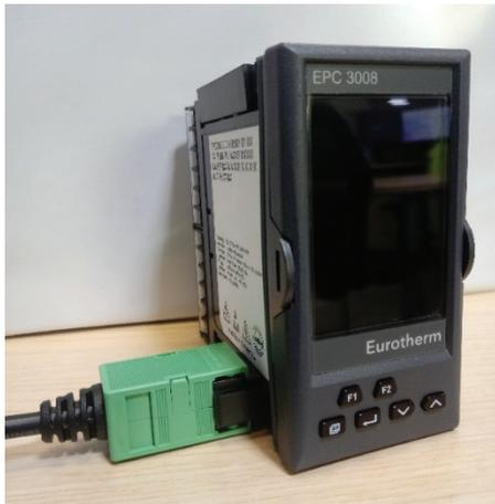
Fig. 12 Controller with connected clip-on connector
