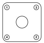
DN15 - DN50 bonnet tightening sequence
