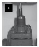
After each tightening sequence lift the stem fully.
