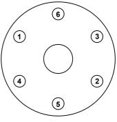
DN65 - DN100 bonnet tightening sequence
