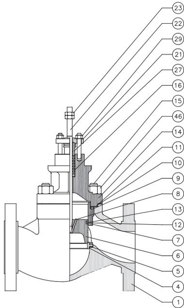
**Fig. 3 - 85 Series with integral flanges**
