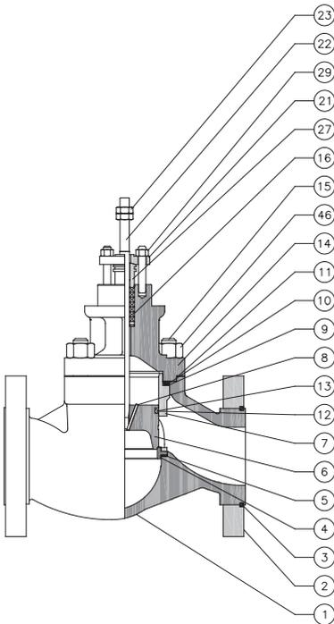
**Fig. 2 - 85 Series with loose flanges**
