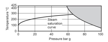
The product **must not** be used in this region or beyond the parameter of the PMA or TMA of the relative end connection.
