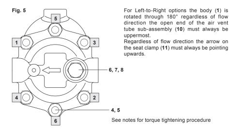
See notes for torque tightening procedure
