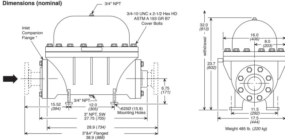
\* The inlet connection on NPT and SW traps is a standard 4" (DN100) ANSI 300 RF Flange bolted to the trap body. The flange bore is 3" (DN80), NPT or SW to match the outlet connection of the trap.
