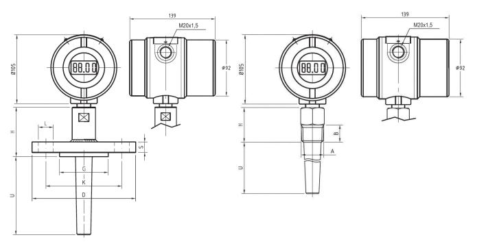
Figg. 1 - TT372 coupled with flanged thermowell
