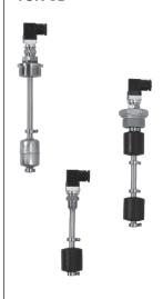
The compact type CD is recommended for applications in hydraulic control units. It can also be used with liquids with low specific weight such as hydrocarbons and mineral oils. The floats are made of stainless steel or BUNA N, the other wetted parts are made of stainless steel. The compact type **CD** can be equipped with reed switch contacts. allowing control of up to two switching points with a single instrument. In place of the housing, a three-pin DIN connector with flying plug is used.
