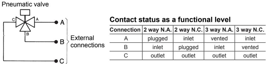
Fig. 4 - Pneumatic switch diagram
