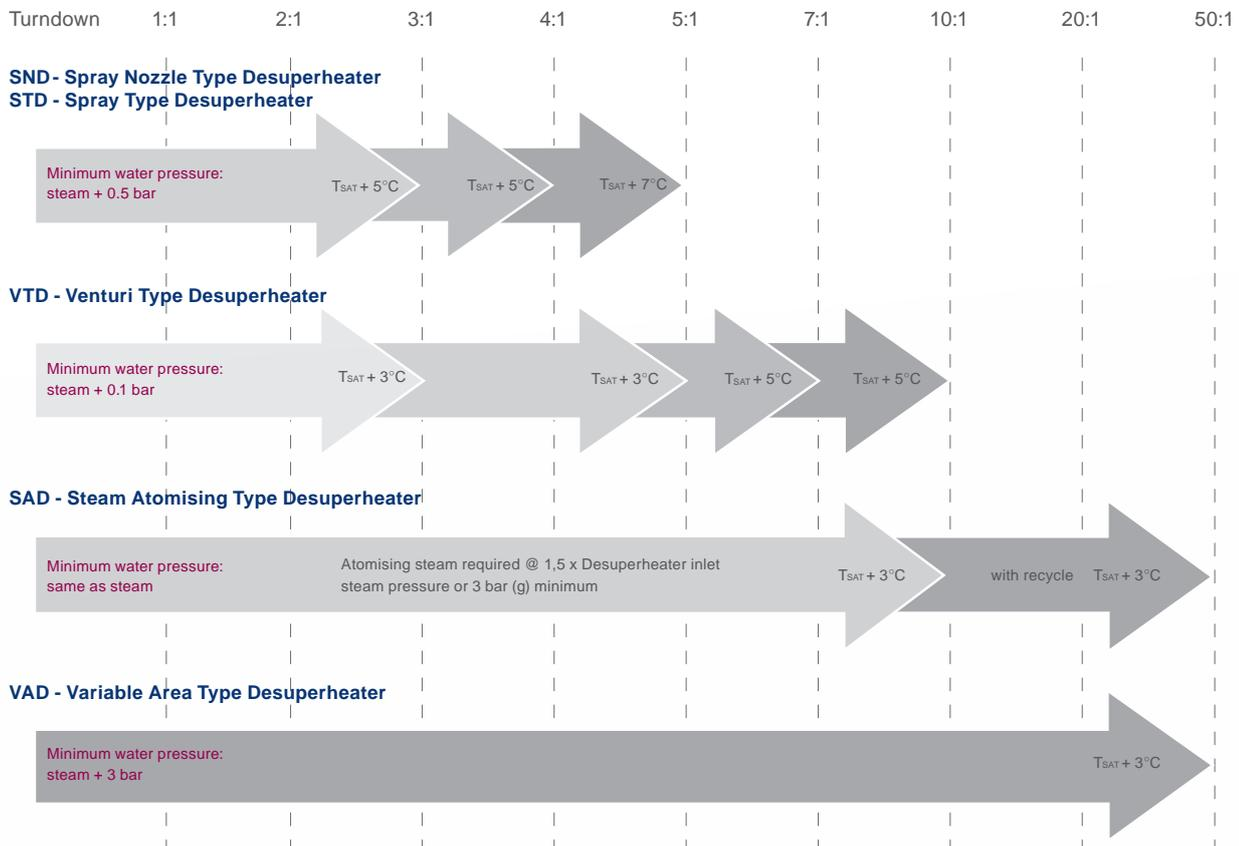
Turndown ratio is dependent on a wide variety of factors, such as, installation (horizontal or vertical), amount of residual superheat, and piping. Dependant on conditions the turndown figures quoted for desuperheaters are the maximum capable
