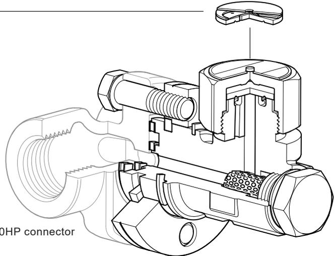
UTD26LY and UTD26HY shown fitted to a PC10HP connector
