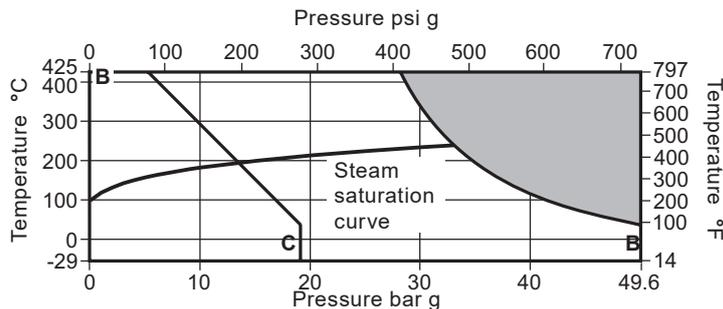
The product **must not** be used in this region or beyond the parameter of the PMA or TMA of the relative end connection.
