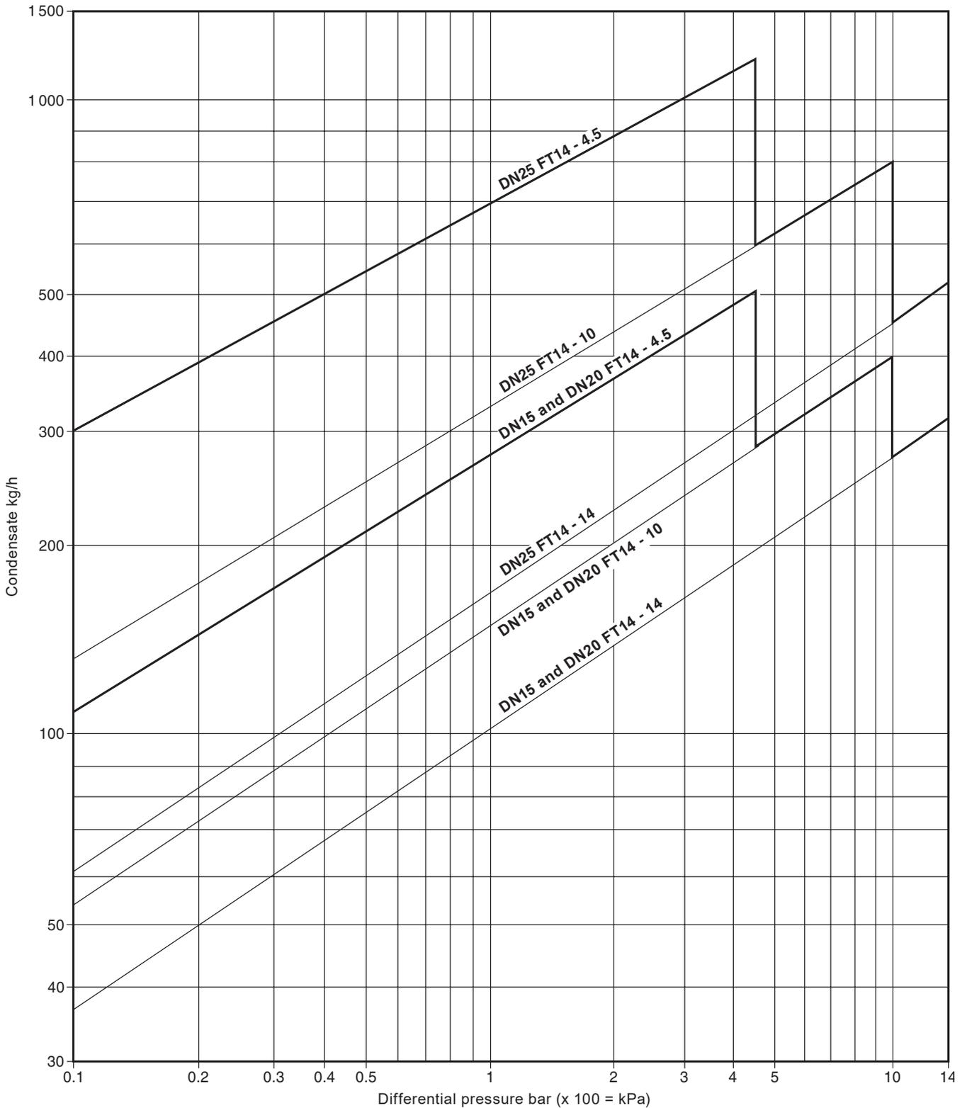
Capacities shown above are based on condensate at saturation temperature. When discharging sub-cooled condensate the air vent provides extra capacity. Under start-up conditions when the condensate is cold the internal thermostatic air vent will be open and provides additional capacity to the main valve.
