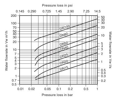
Pressure loss diagram with open valve at 20 °C (68 °F). The values indicated are applicable to spring loaded valves with horizontal flow. With vertical flow, insignificant deviations occur only within the range of partial opening.
