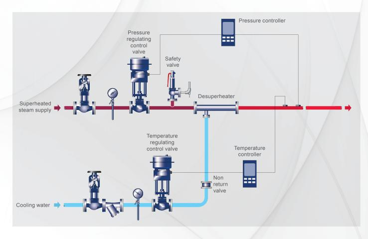
A typical desuperheater installation will require isolation valves for both the steam and cooling water pipelines. The BSA3HP is the ideal solution for use on ASME Class 600 rated desuperheater packages.
