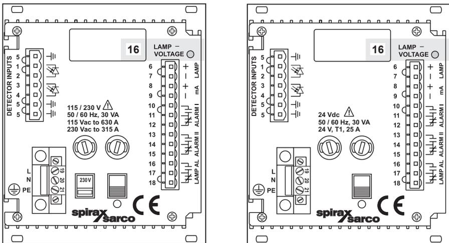
Fig. 19 Potentiometer for lamp voltage
