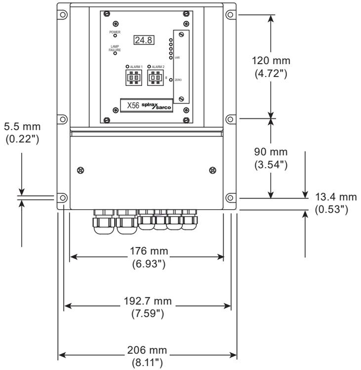
**Fig. 5 Dimensions with wall mount housing B19-21**
