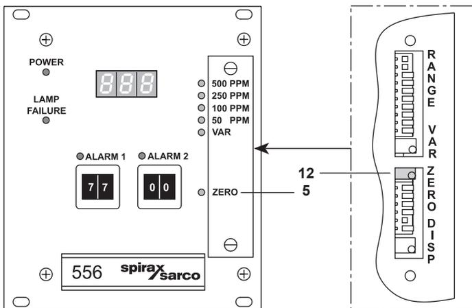
Fig. 20 Potentiometer for zero point setting
