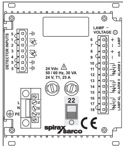
Fig. 10 Power switch on converter 115/230 V (left) and 24 V (right)
