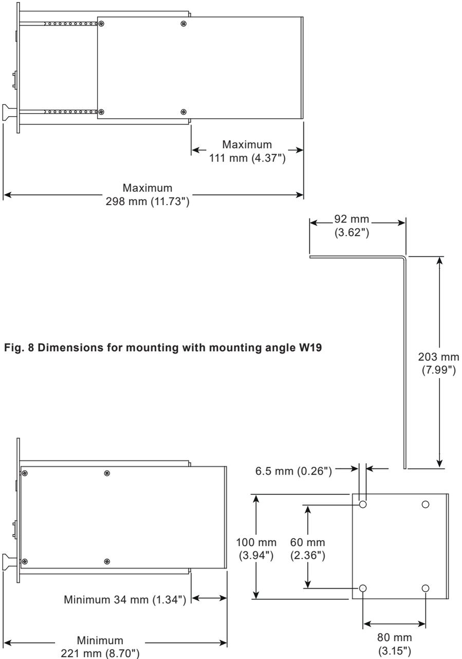
**Fig. 8 Dimensions for mounting with mounting angle W19**
