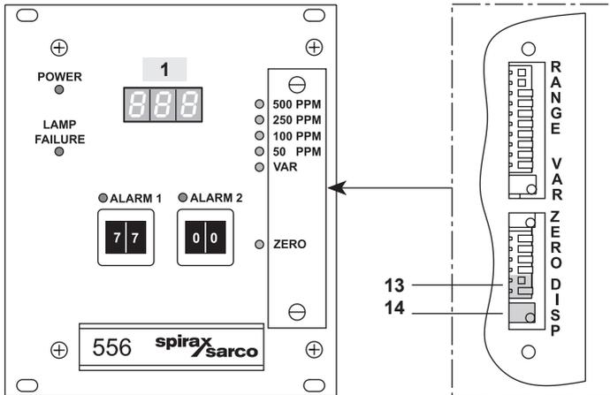
**Fig. 23 Potentiometer for digital read-out adjustment**
