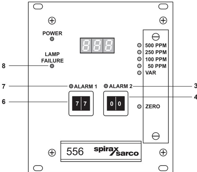
Fig. 22 LEDs and encoding buttons for alarms
