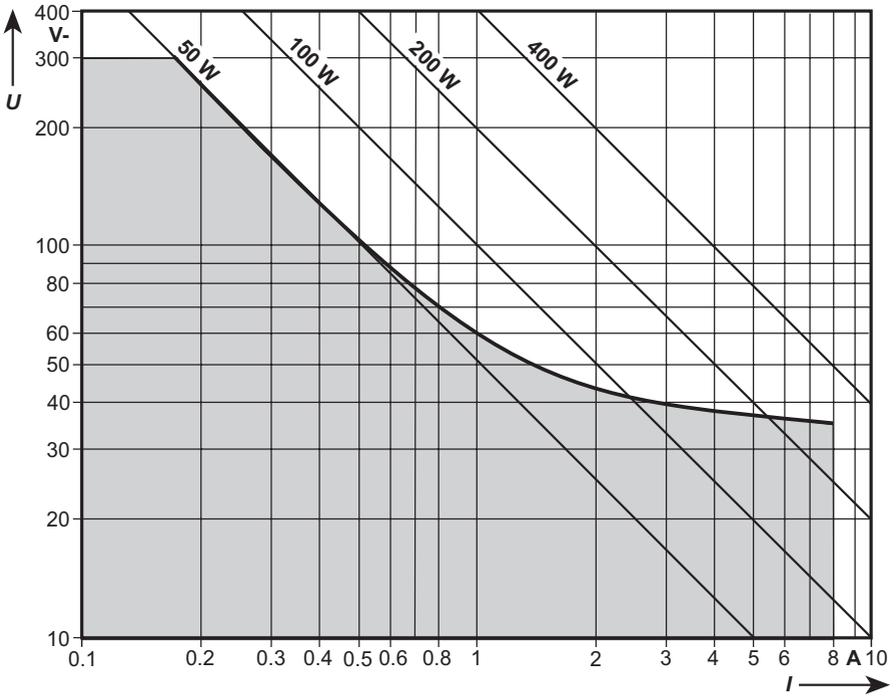
Fig. 16 Load limit curve relay outputs
