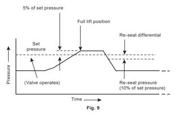
It can be seen that the safety valve does not re-seat when the pressure falls to the safety valve set pressure. There must be adequate differential between the maximum system operating pressure and the safety valve set pressure if the valve is to re-seat.
