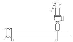
8 - 10 pipe diameters downstream of converging 'Y' fittings or bends.
