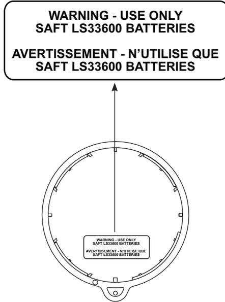
Fig. 25 Label inside the battery compartment (back of the front cover)
