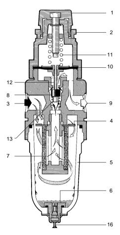
Any appreciable rise in the secondary pressure from its set value will cause the diaphragm and the push rod (12) to lift. This will allow air to escape through the centre of the push rod to atmosphere. When excess pressure has vented, the orifice in the push rod will reseat on the main valve
