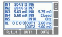
At the top of the screen are displayed the signals on the activated inputs. At the bottom left are showed output relays status (O = open, C = closed), and at the right current outputs 4-20 mA (---- means that the output is off). Black color of inscriptions indicates that the state is not a result of normal operation of the device, but was forced for the test. To enforce the desired states of the output relays press **RL1..4**.
