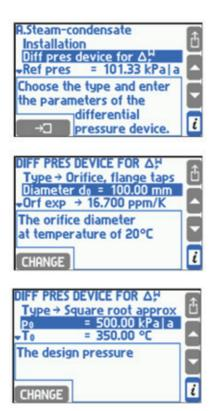
According to PN-EN ISO 5167 standard one of differential pressure devices can be chosen one of standard primary flow devices:
