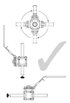
Fig. 4 Correct installation for gas service
