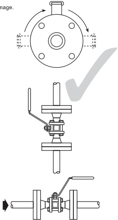
**Fig. 3 Correct installation for gas service**
