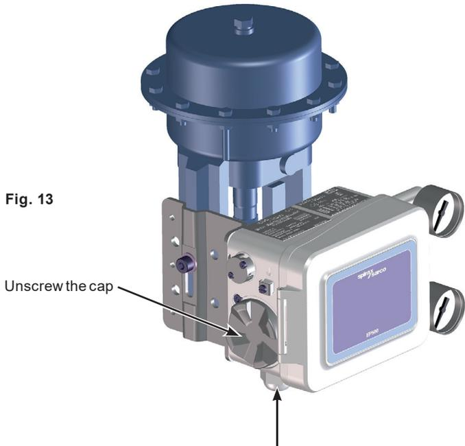
Insert the electric cable (4 to 20 mA), connect to the appropriate terminals and screw the cap.
