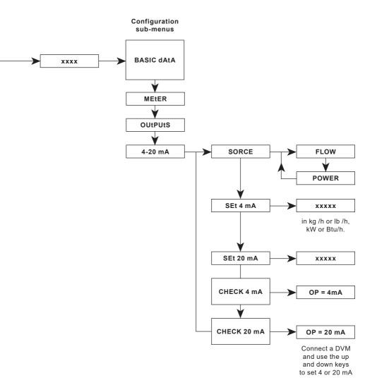
From the Basic dAtA menu navigate to OUtPUts and press the right arrow to enter the sub menu of 4 - 20 mA.
