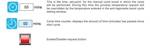
Finally the unit must be manually enabled from the enable request pushbutton located on the HMI, the user can stop the anti-legionella boost cycle at any time by pressing the same button.
