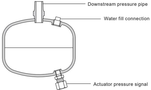
Fig. 2 Water seal pot - WS4/WS4-3
