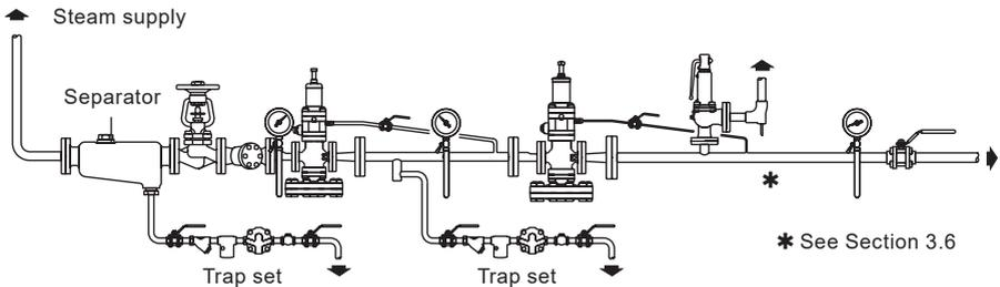
Fig. 6 Two pressure reducing valves installed in series
