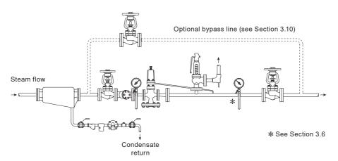
Fig. 5 Setting procedure sequence DP163, DP163G and DP163Y
