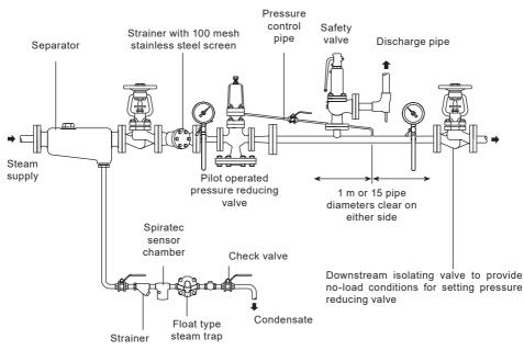
Fig. 2 Recommended installation
