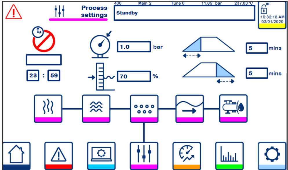
Main process set-points (400). Including clean steam pressure, water level, ramp up time and ramp down time.
