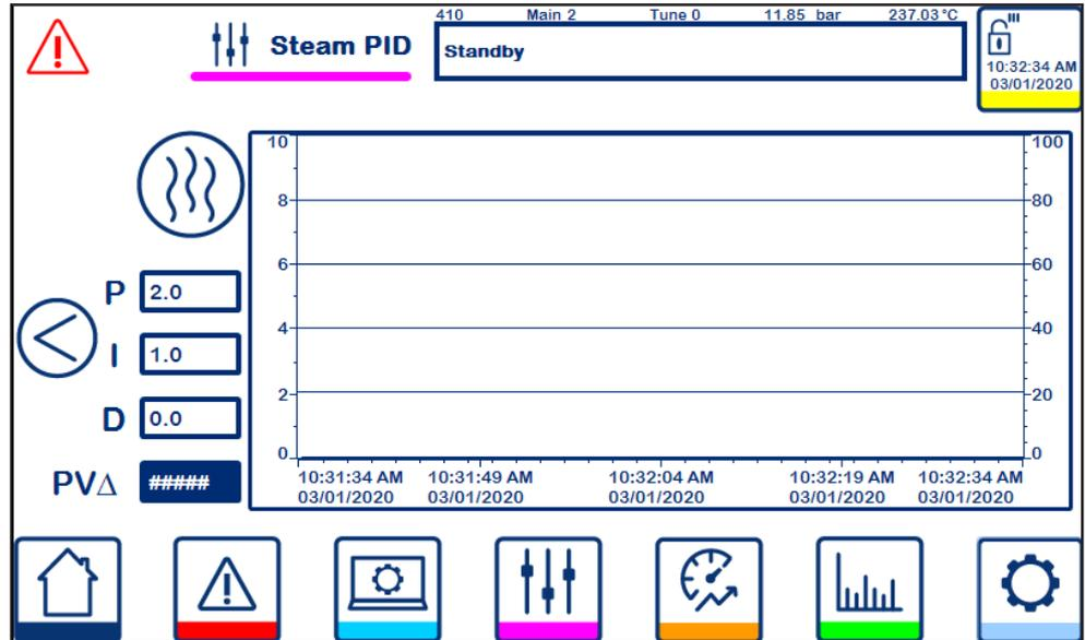
Steam PID settings (410) also includes a live PID graph showing the process and control values, and the process set-point.
