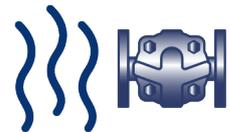
The Trap Failed Open alarm when a preheater is not fitted is triggered when the control valve is only open a small amount, and the condensate temperature sensor TA51 and the drain temperature sensor TA52 are similar temperatures.
