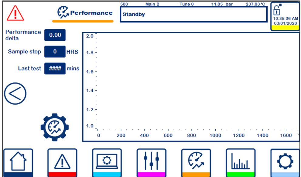
Performance data (500), as well as showing the current performance profile of the CSG-HS also shows the current data sample and data times.
