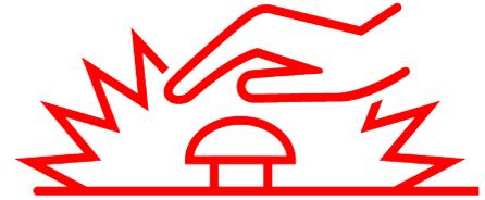
When the emergency stop is triggered, the status of the CSG-HS is changed directly to 'Emergency Stop', overriding any previous run status. Additionally, all automated isolation valves are reset, control valves are closed and the water pump (if fitted) is disabled.
