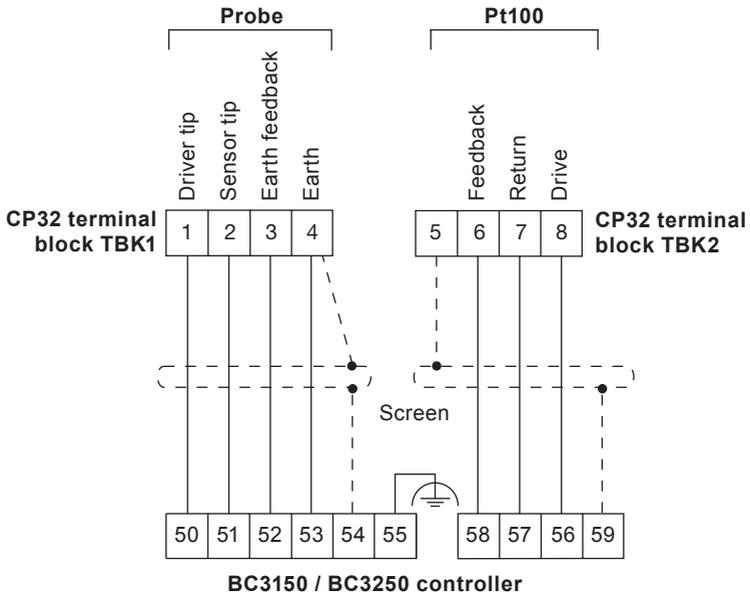
Ensure resistance from probe body to pipework/boiler shell is less than 1 Ω.
