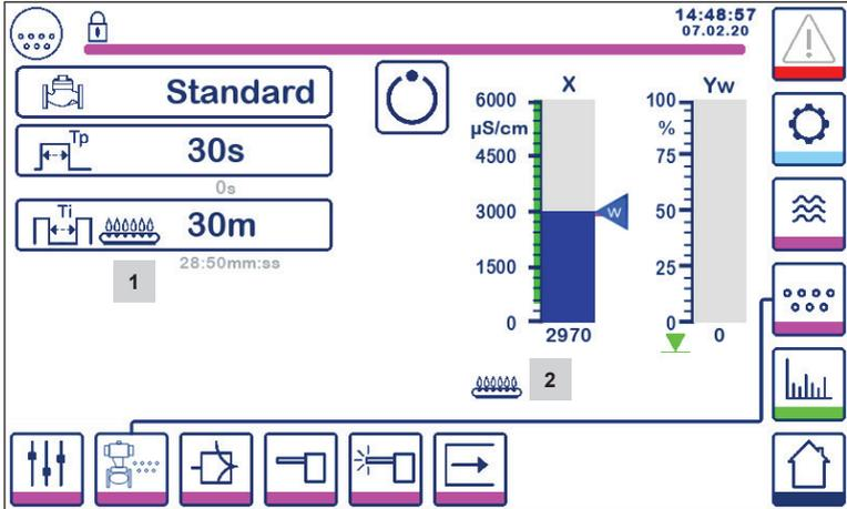
Fig. 29 Purge setup for ON/OFF control - burner input
