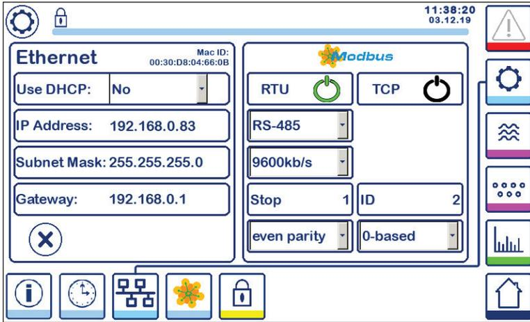
Fig. 46 Modbus RTU protocol
