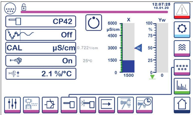
Fig. 34 Temperature compensation
