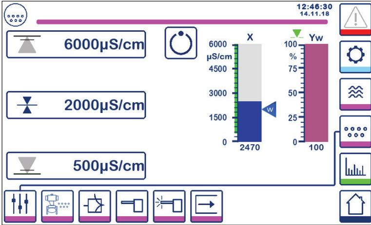
Fig. 23a Modulating control (VMD)
