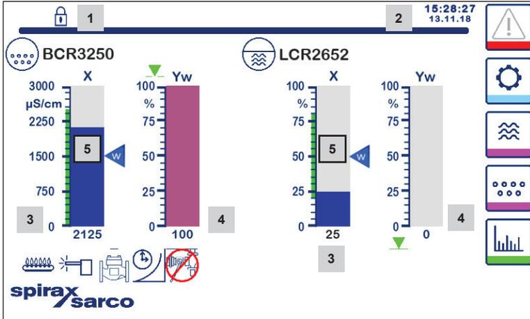
Fig. 22 Start window (with BCR3250 and LCR2652 fitted)
