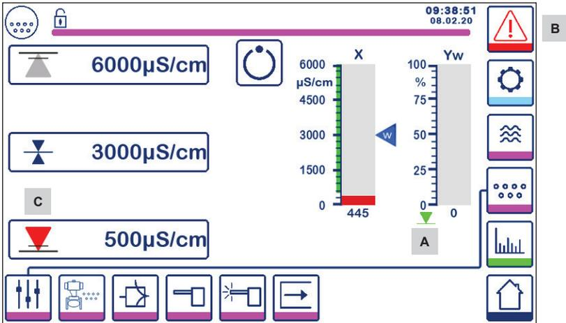
Fig. 51 TDS/Conductivity MIN alarm
