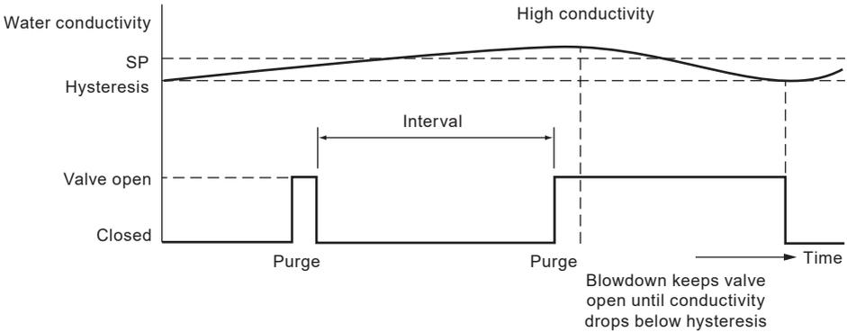
Fig. 17 ON/OFF control with purge
