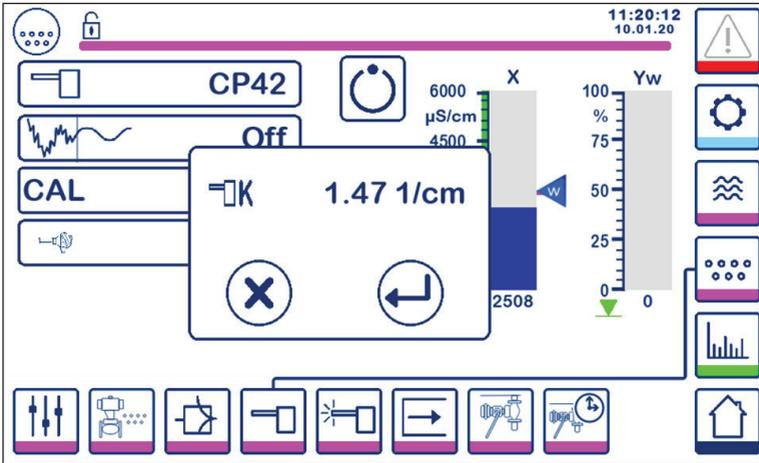
Fig. 35 Calibration with probe in boiler
