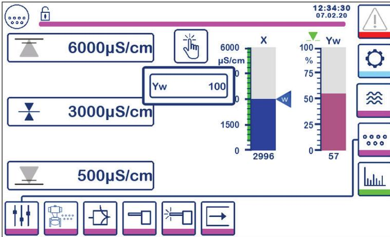
Fig. 26a Modulating control (VMD)
