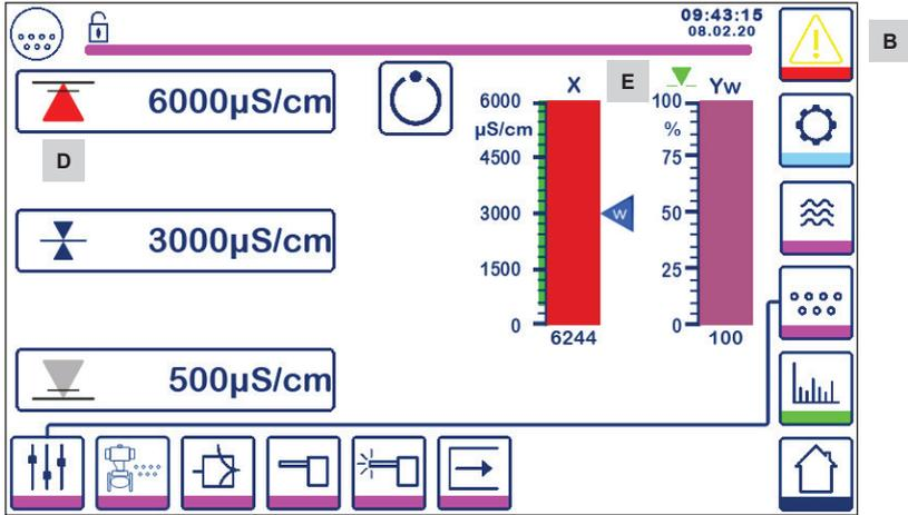
Fig. 52 TDS/Conductivity MAX alarm
