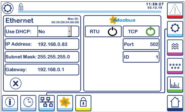
Fig. 45 Modbus TCP settings
