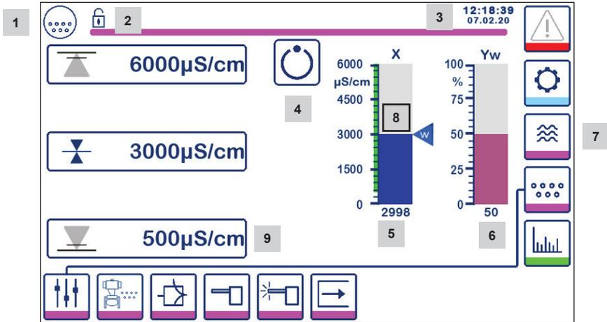
Fig. 21 Start window (without LCR2652 fitted)
