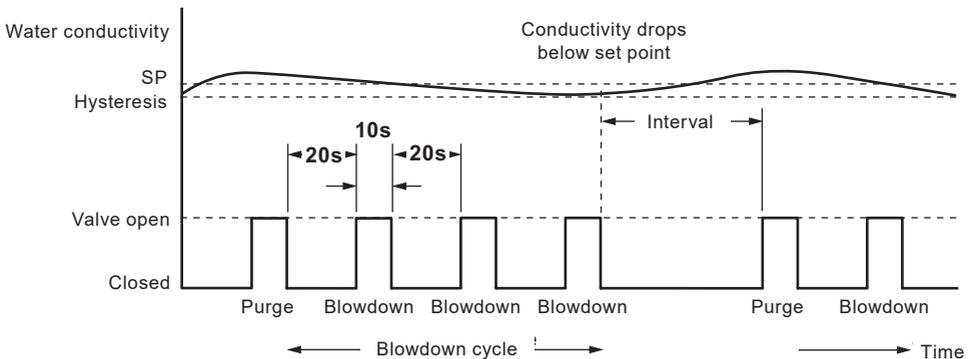
Fig. 18 ON/OFF control with purge and pulsed output
