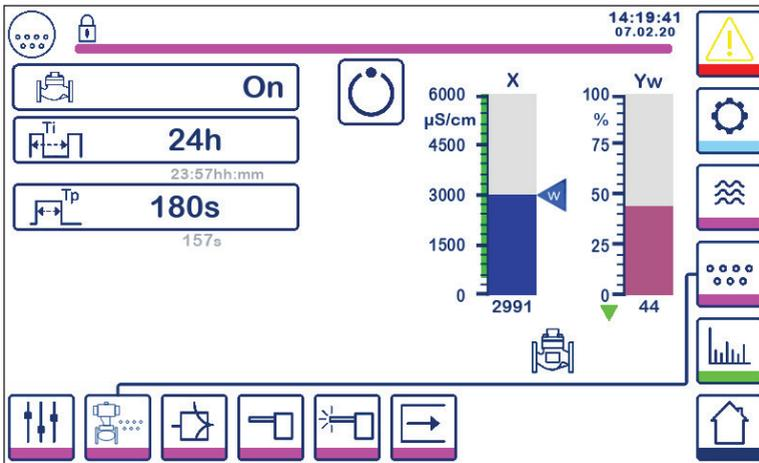
Fig. 27 Rinsing setup for modulating control (VMD)
