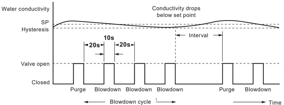
Fig. 21 ON/OFF control with purge and pulsed output
