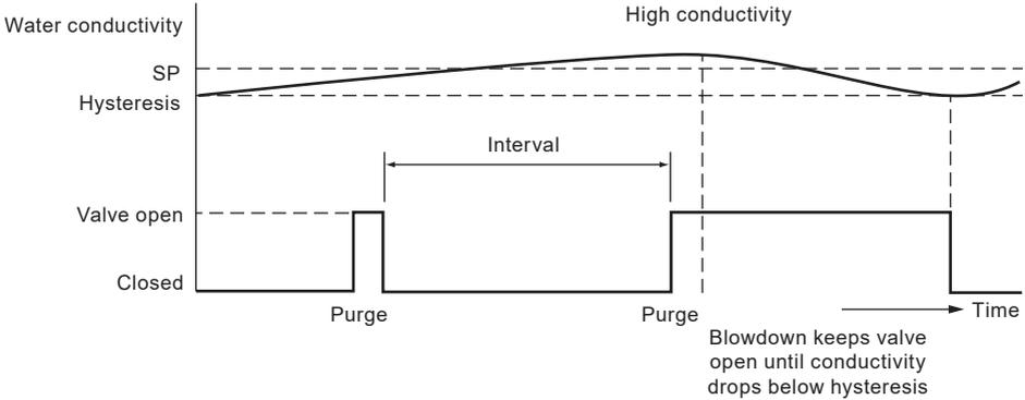
Fig. 20 ON/OFF control with purge
