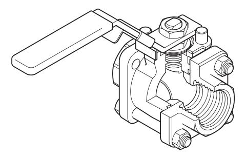
**Description**The M10Pi ISO three-piece body ball valve has been designed for use as an isolating valve, not a control valve, has a lockable handle as standard and can be serviced without removal from the pipeline (screwed and welded versions only). It can be used with process fluids for services ranging from vacuum to the higher temperatures and pressures.
