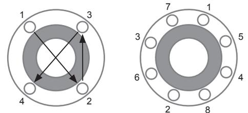
Flange bolts should be gradually tightened across diameters to ensure even load and alignment.
