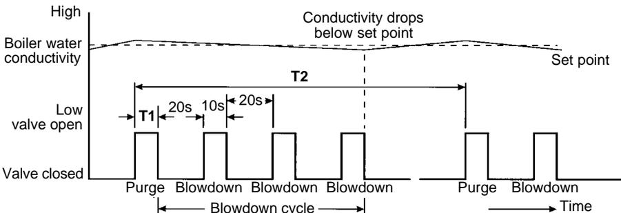
Fig. 3 Conductivity being controlled near to set point
