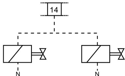
Alternative arrangement for two 2-port valves
