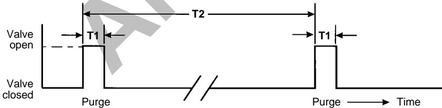
Fig. 2 Measured conductivity lower than the set point
