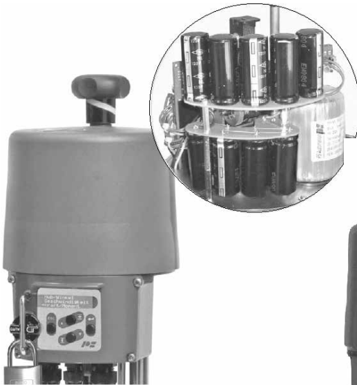
Fig. 14 Internal super capacitor for the following actuators: AEL62_, AEL63_, and AEL64_
