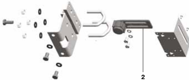
Fig. 4 Pillar mounting kit for a linear actuator
