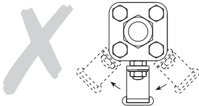
**Fig. 2 Incorrect installation for liquid service**
