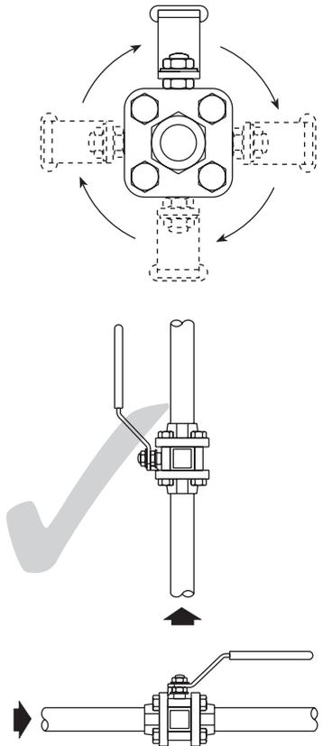
**Fig. 3 Correct installation for gas service**
