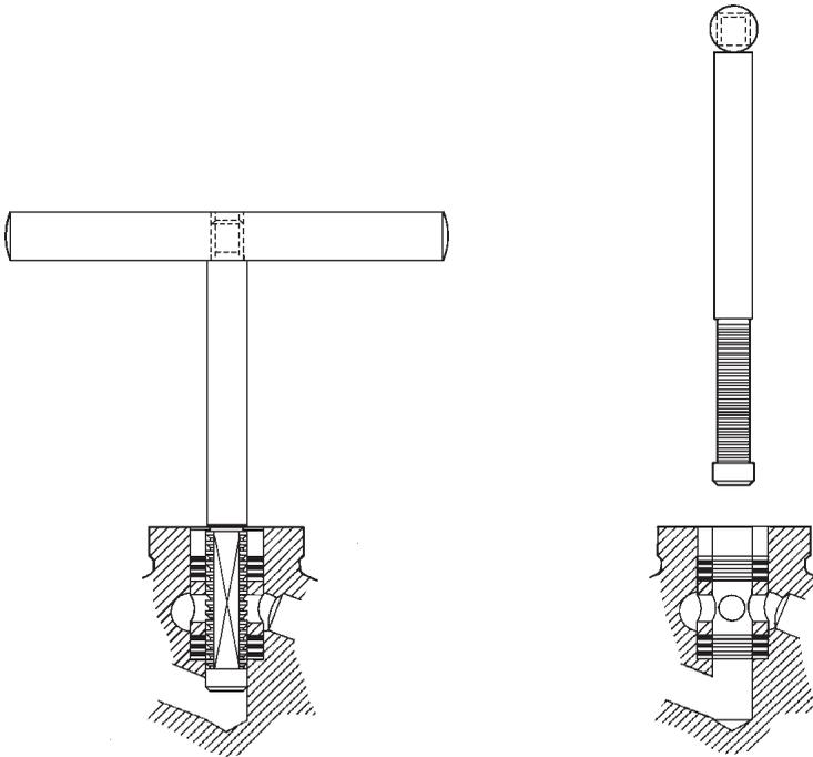
Fig. 4 View showing valve internals extractor tool
