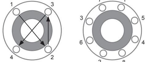
Flange bolts should be gradually tightened across diameters to ensure even load and alignment.
